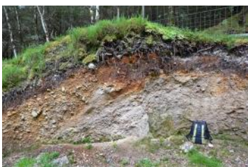
Photograph 3: A small roadside quarry (or 'borrow pit') which provides a convenient cross section showing grass and moss growing on a thin layer of black forest peat, which overlies glacio-fluvial deposits which overlie
